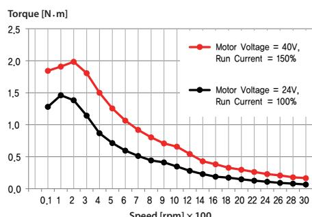
\* The torque at low speed and high speed is improved about 30%.
