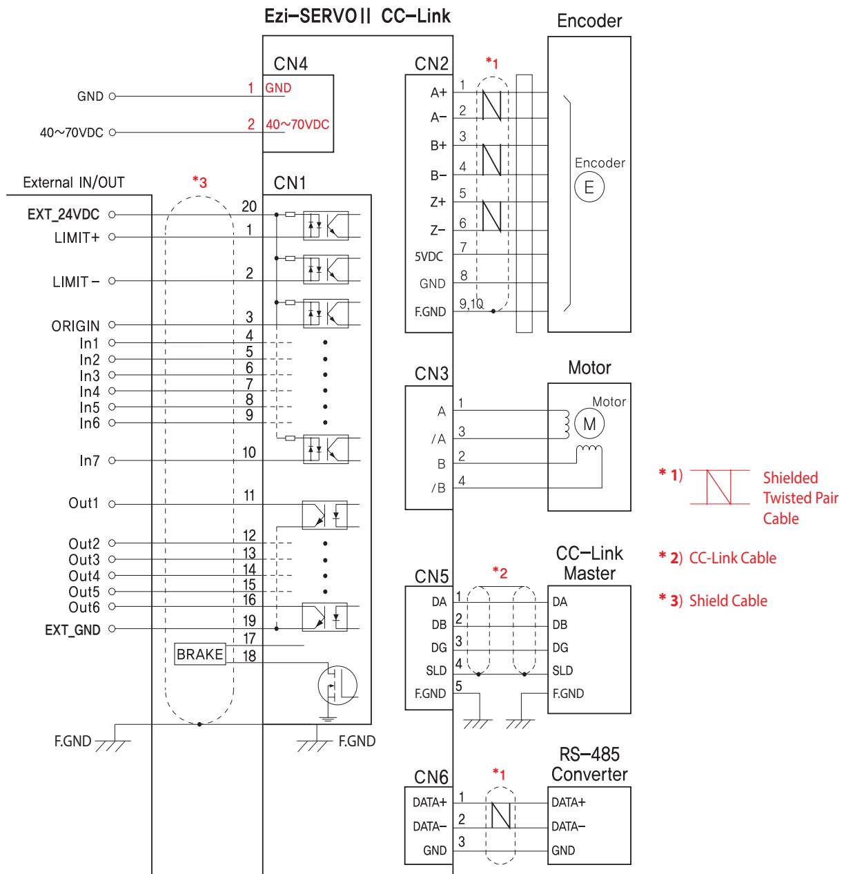
※ When connects I/O cable between controller and drive, please turn off the power of both controller and drive, in order to protect the drive from any damage.
