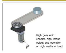
Super HG Series offers high gear ratio as 1:20, 1:36 for model SHG170 and 1:18 for model SHG130 so it enables to drive high inertia of load with very strong output torque from hollow rotary table, Also high gear ratio enables minimization of load inertia moment ratio so it realizes smooth operation at Acceleration/Deceleration and no hunting when it stops suddenly.
